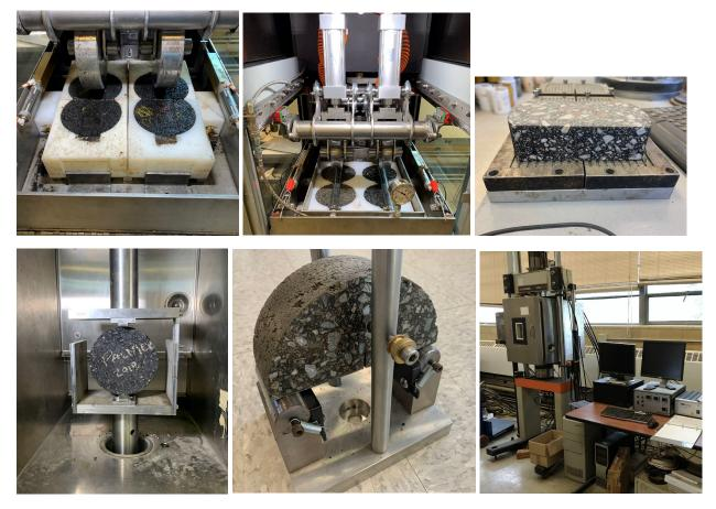
Figure 4-2 Mixture Performance Testing conducted at the CAP Lab in preparation for Balanced Mix Design Implementation. Clock-wise from the top-left corner: Hamburg Wheel Tracker (AASHTO T324), Asphalt Pavement Analzyer (AASTO T340), Texas Overlay Test, 100 Kn Instron 1331 Load Frame with FastTrack 8800 Data Acquistion System, SCB-FIT Test (AASHTO TP-124), IDEAL CT Cracking Test (ASTM D8225)
