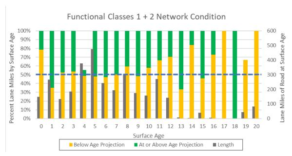
Figure 2-12 PSPI Ranking at or above projected condition level vs. age for Functional Classes 1 and 2
