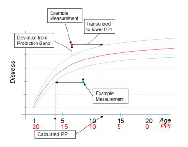
Figure 2-10 Concept Level Graphic for PSPI Model Determination
