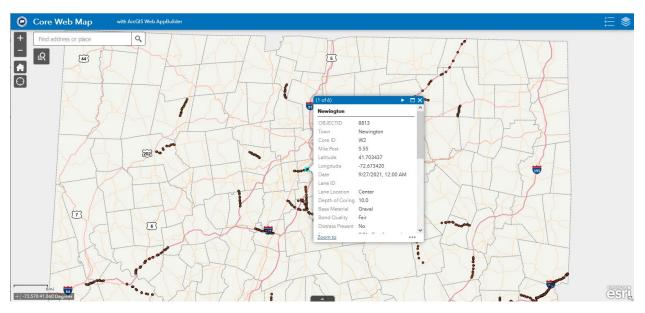
Figure 4-3 Core Database for State-wide Forensic Pavement Coring in the TED/GIS Interface
