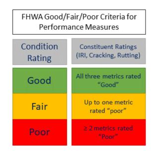
Figure 2-14 FHWA Performance Measure Criteria for Good/Fair/Poor Ratings
