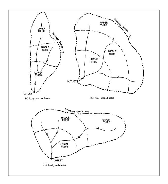
Schematic of typical drainage basin shapes and subdivision into basin thirds. Note that stream-channel distances within any given third of a basin in the examples are approximately equal, but between basin thirds the distances are not equal, to compensate for relative basin width of the thirds.
