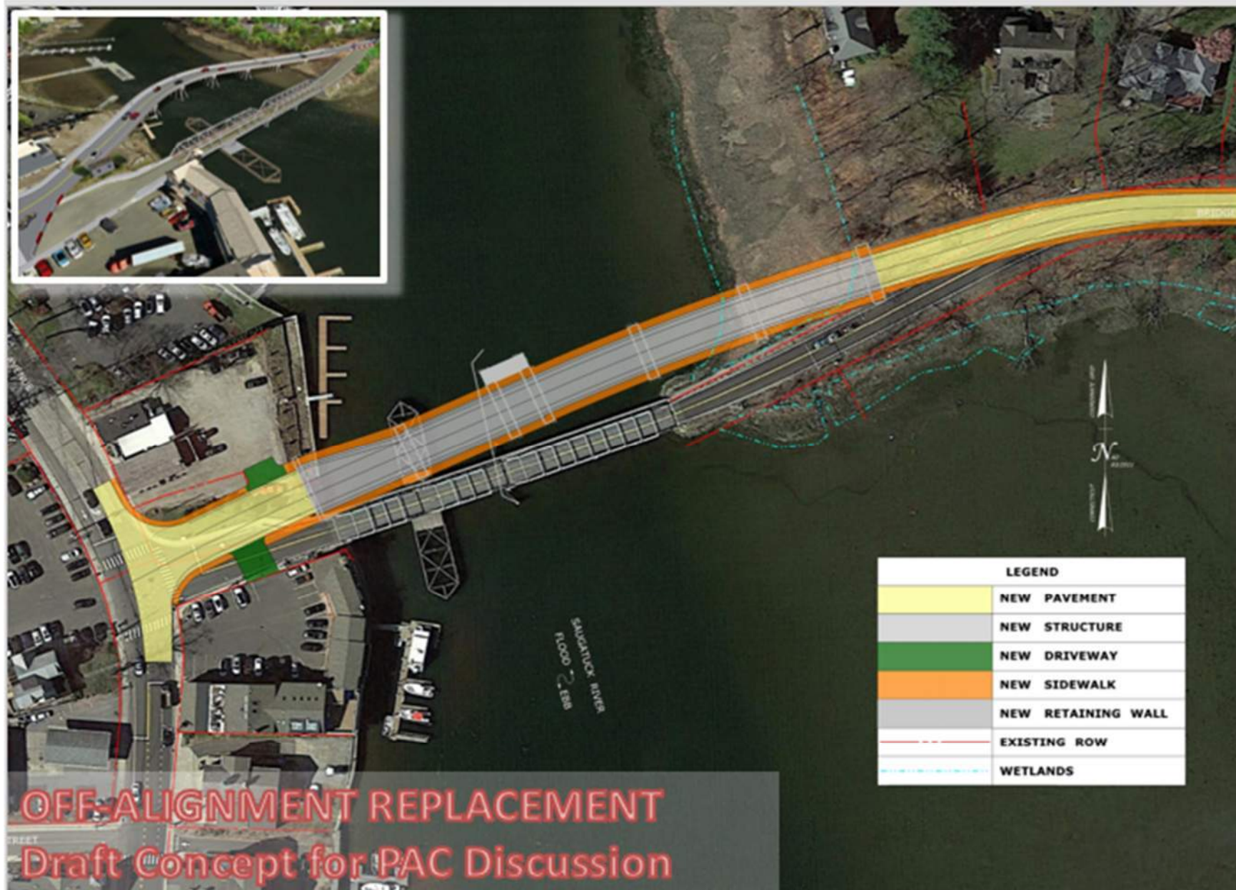
Figure 7: Conceptual plan of Off-Alignment Replacement Alternative. The inset image shows the detour bridge required by the other three alternatives.
