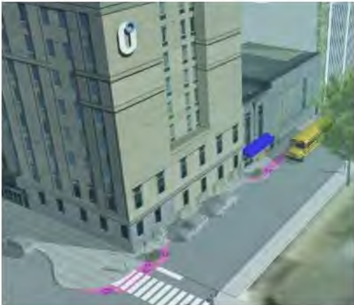
Exhibit 5: Proposed bus loading zone on Bell Street and crosswalk enhancements at the intersection of Washington Boulevard and Bell Street
