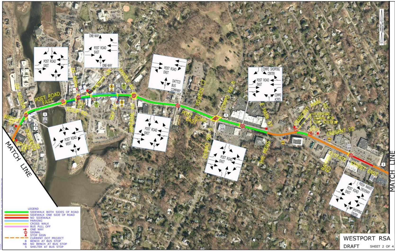
Figure 6. Post Road East, Westport Route 1 - Road Geometrics
