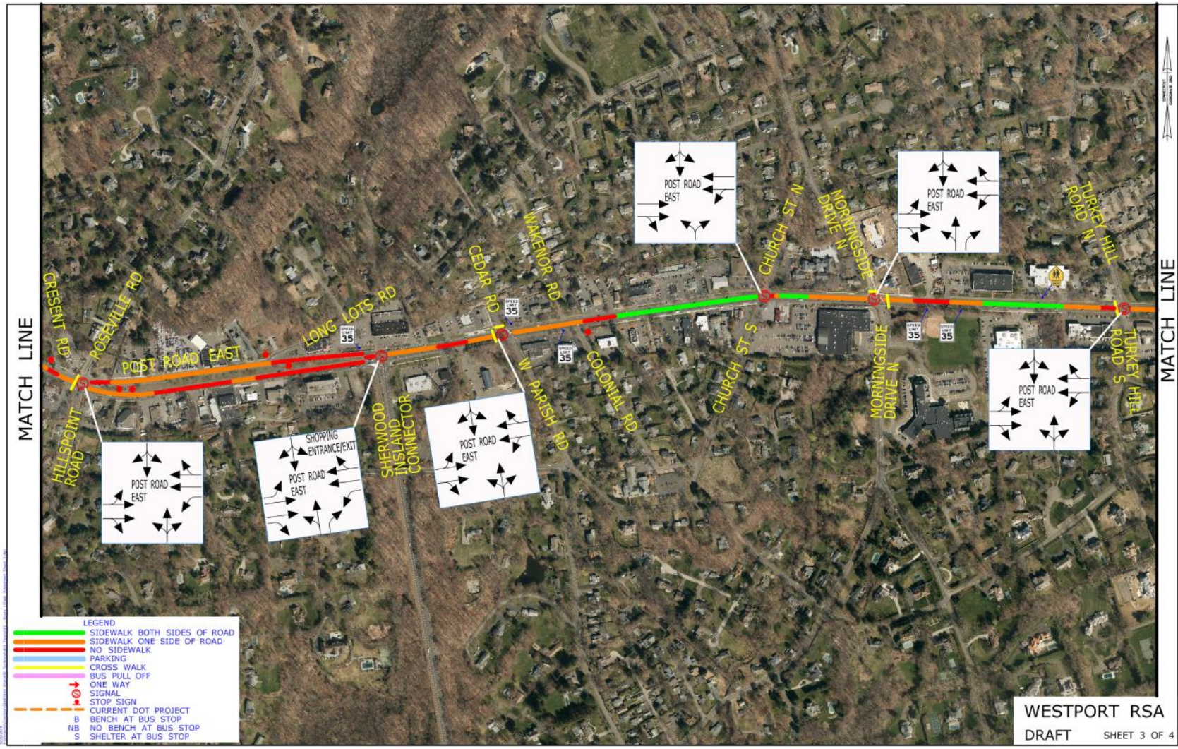
Figure 7. Post Road East, Westport Route 1 - Road Geometrics
