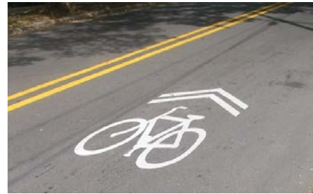
Figure 24. Example of a Sharrow
