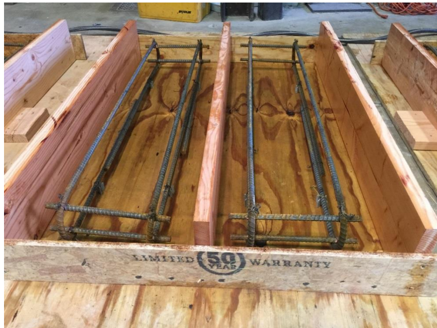
Figure 55. Negative bending flexural test formwork for substrate concrete placement
