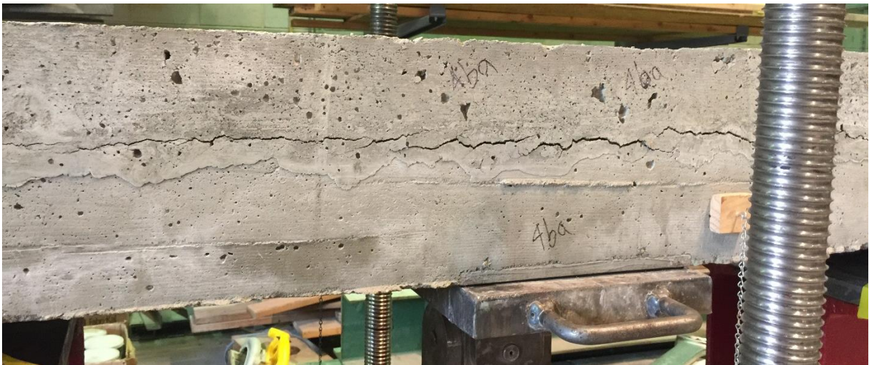
Figure 50. Case 4 positive bending flexural test specimen failure at concrete bond interface
