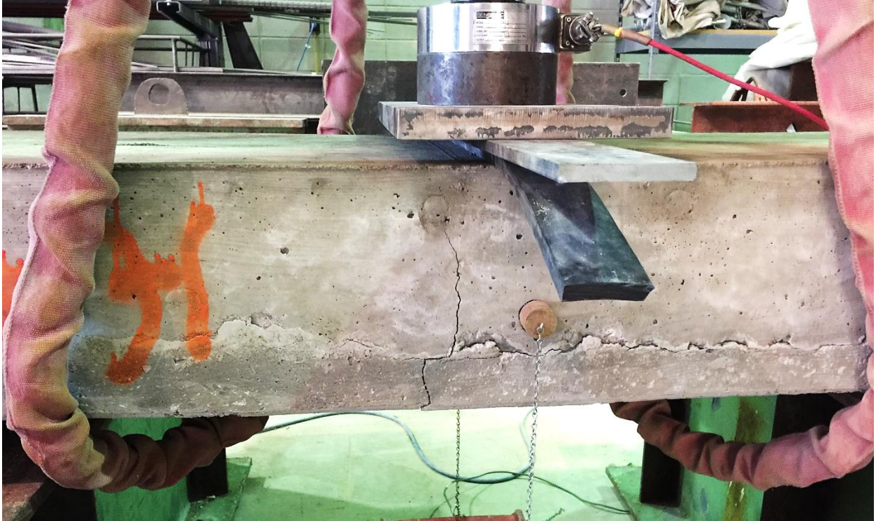
Figure 60. Case 1 negative bending flexural test specimen failure at concrete bond interface
