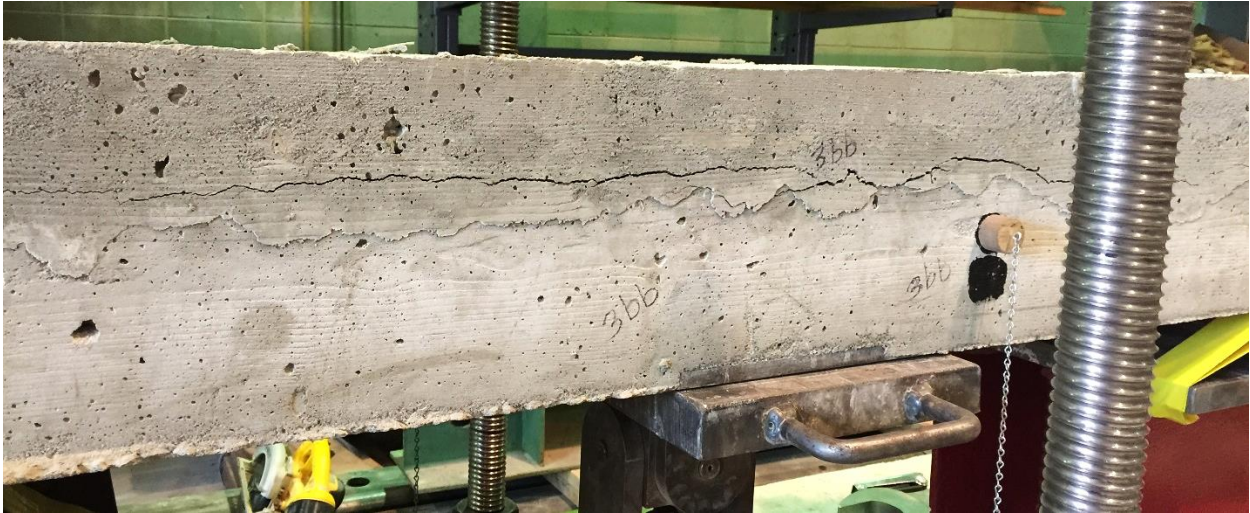
Figure 49. Case 3 positive bending flexural test specimen failure at concrete bond interface
