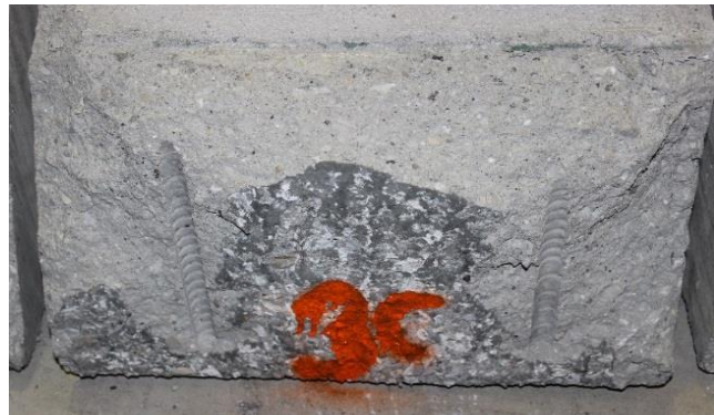
d) Bond interface (overlay concrete)
