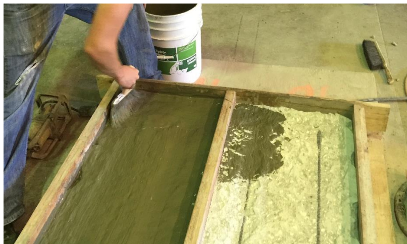
Figure 58. Application of grout to negative bending flexural test specimen
