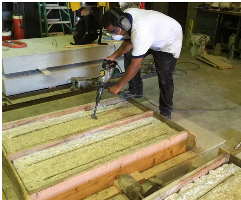
Figure 56. Chipping of substrate concrete for negative bending flexural tests
