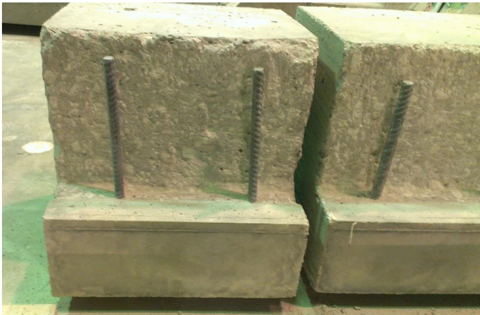
Figure 28. Pair of push-out test sub-specimens after concrete removal (Case 4)
