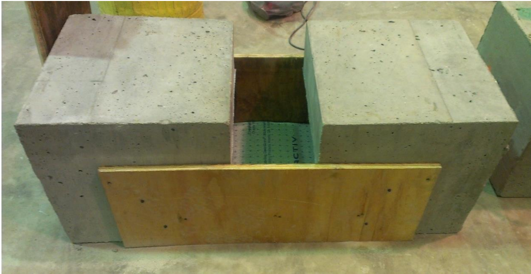
Figure 29. Push-out test formwork for overlay concrete placement
