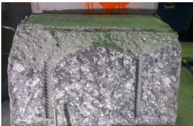
d) Bond interface (overlay concrete)
