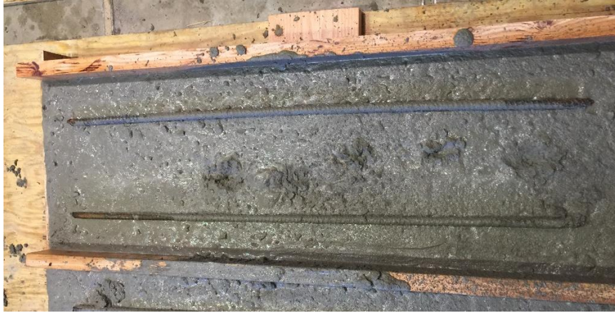
Figure 43. Positive bending flexural test specimen after substrate concrete placement (Case 4)
