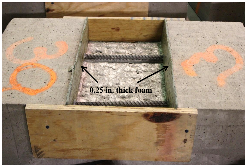
Figure 12. Pull-off test formwork for overlay concrete placement (Case 4)
