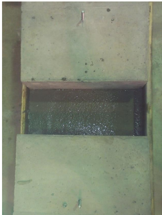
Figure 31. Push-out test specimen after overlay concrete placement
