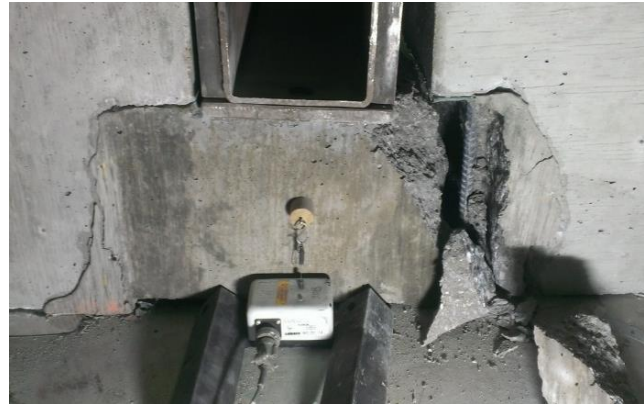
b) Separation at interface
