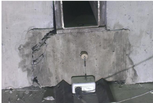
b) Separation at interface
