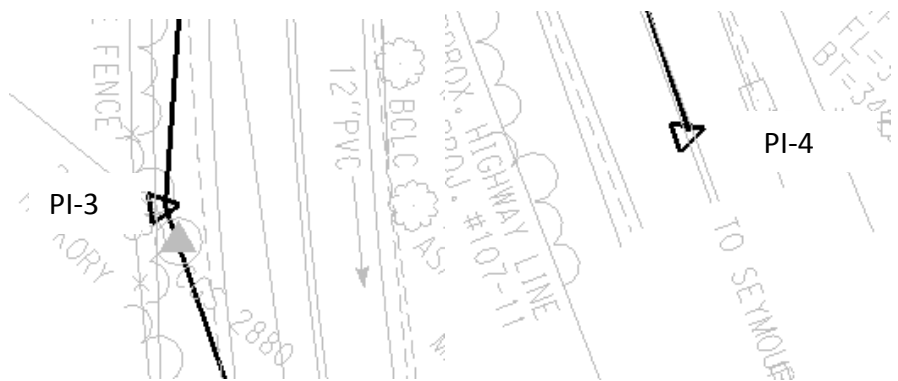
Figure 4-3 Mainline Horizontal PI Point Locations
