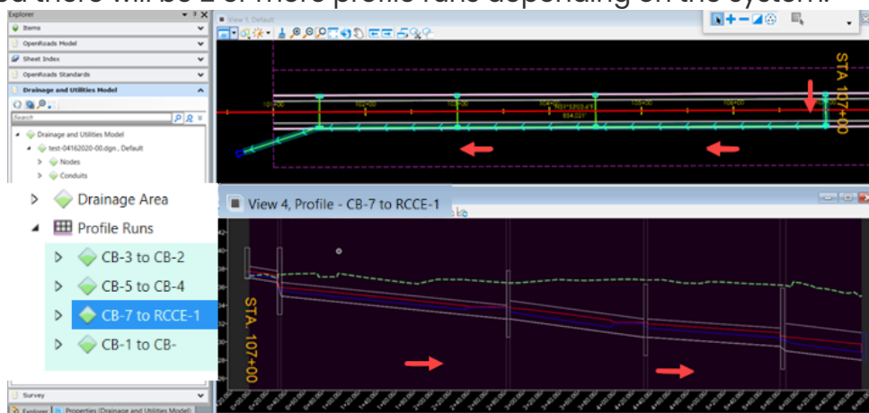
Figure 78 Hydraulic Run To Outfall
