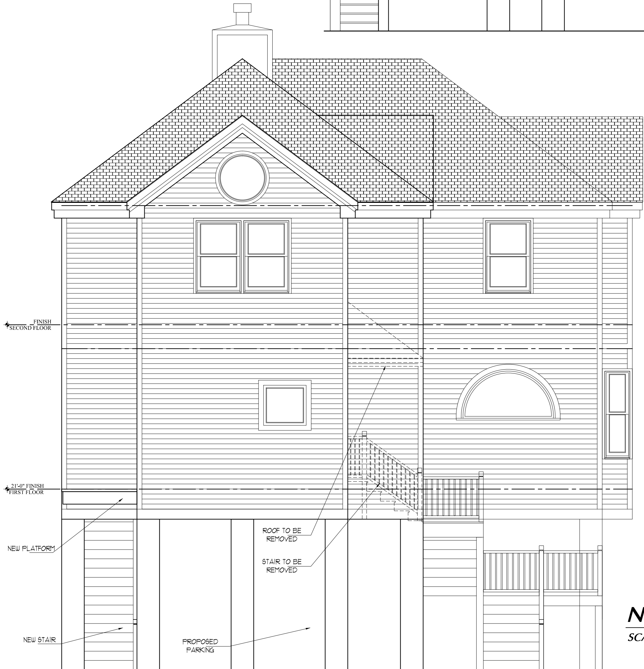
EAST ELEVATION SCALE: 1/4"=1'-0"
