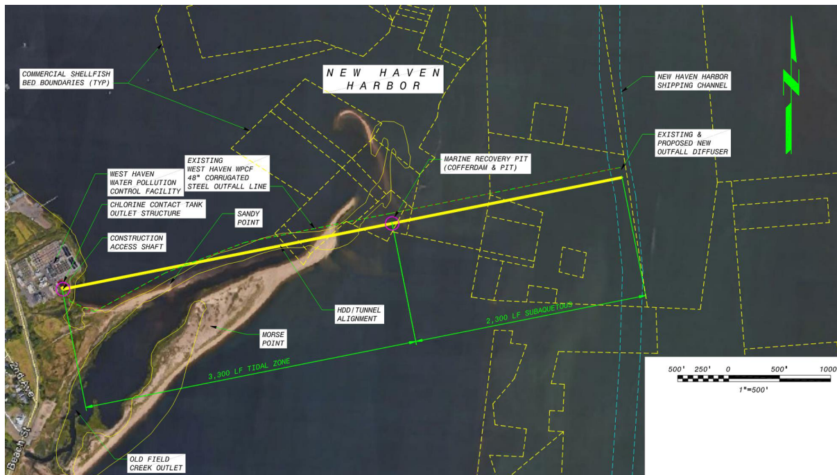
Figure 6 Outfall alignment for HDD or Tunneling Alternatives
