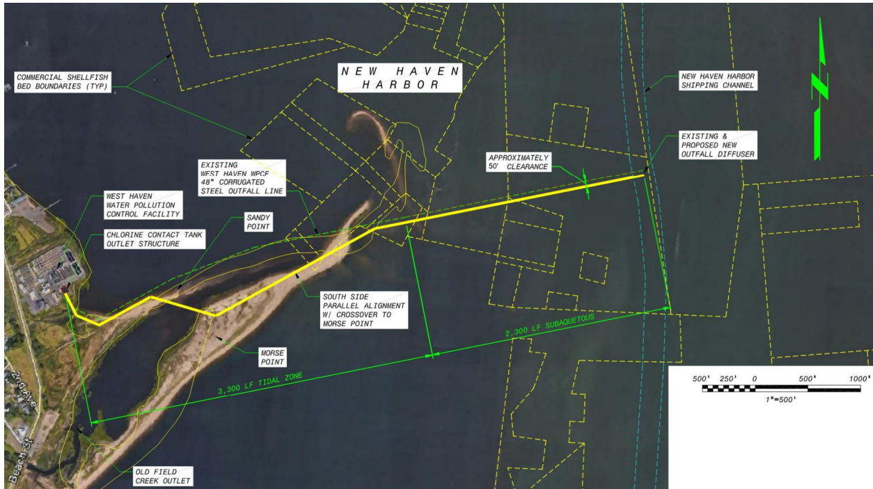
Figure 4 Outfall alignment with crossover to Morse Point
