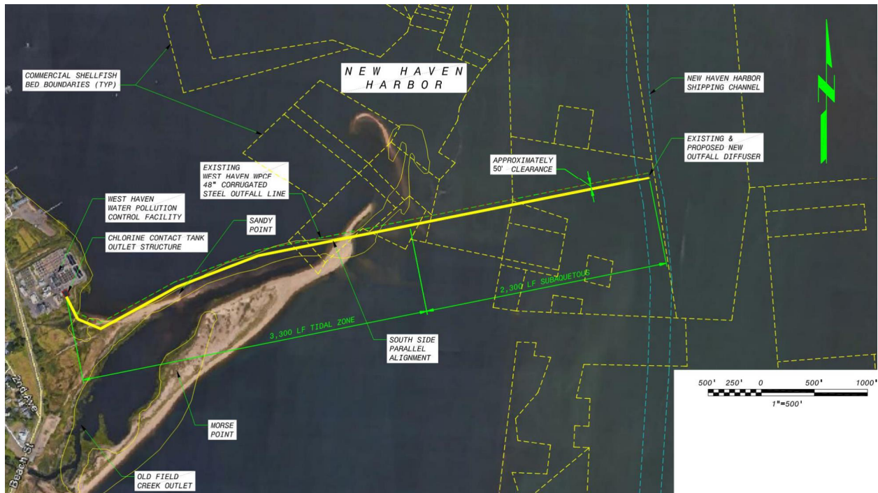
Figure 3 Outfall alignment, south of existing alignment.
