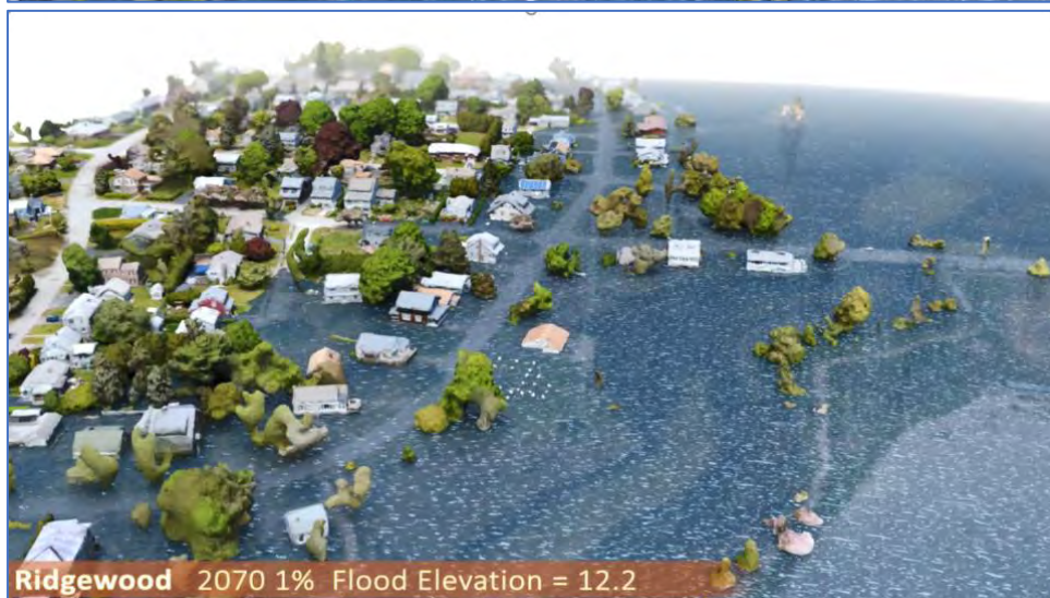
Figure 6 - Ridgewood Area Looking North Along Shore Drive – 1% (100 Year) Coastal Floods
