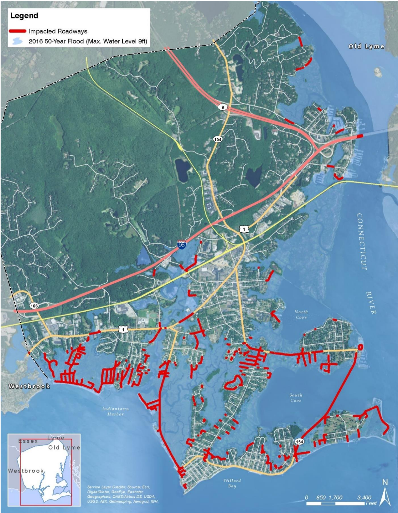
Figure 4-39: Current 50-year Recurrence Interval Flood Risk Roadway Inundation
