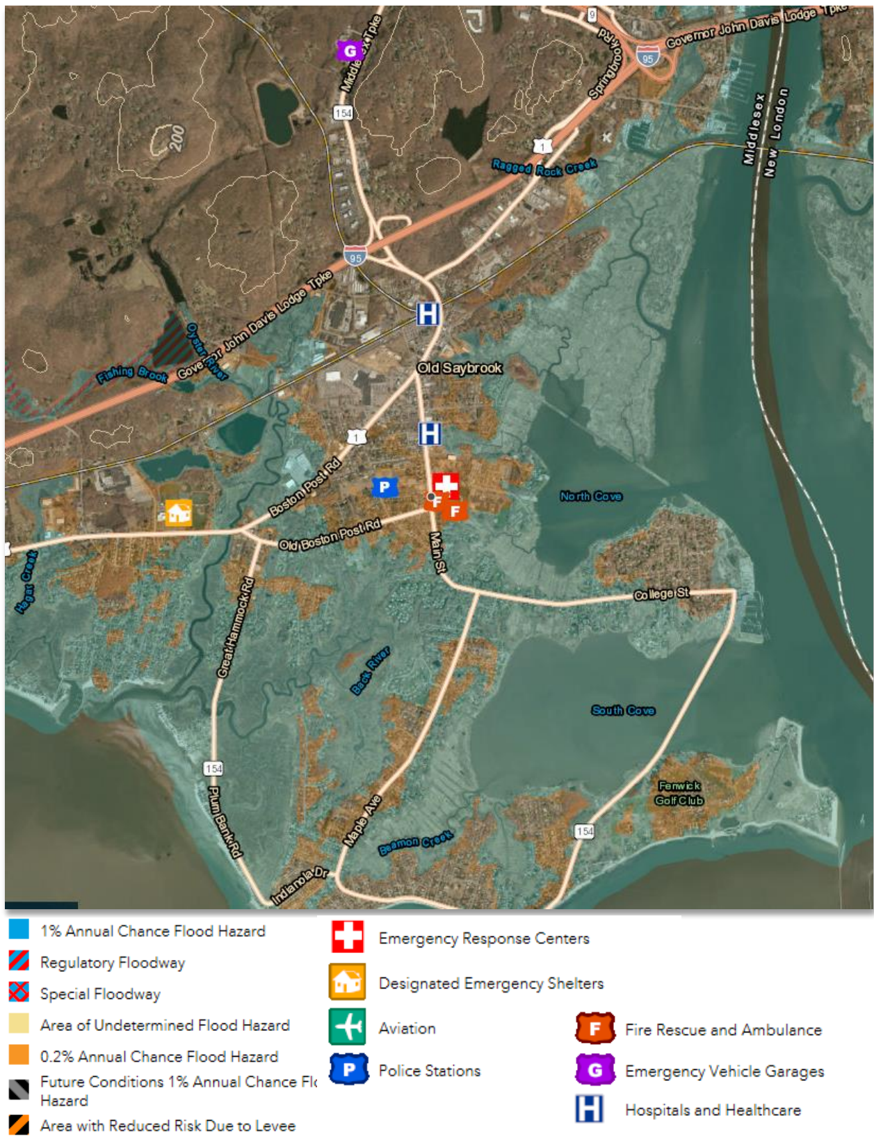
Figure 4-18 Location of Essential Facilities relative to Predicted Coastal Flood Limits FEMA FIRM
