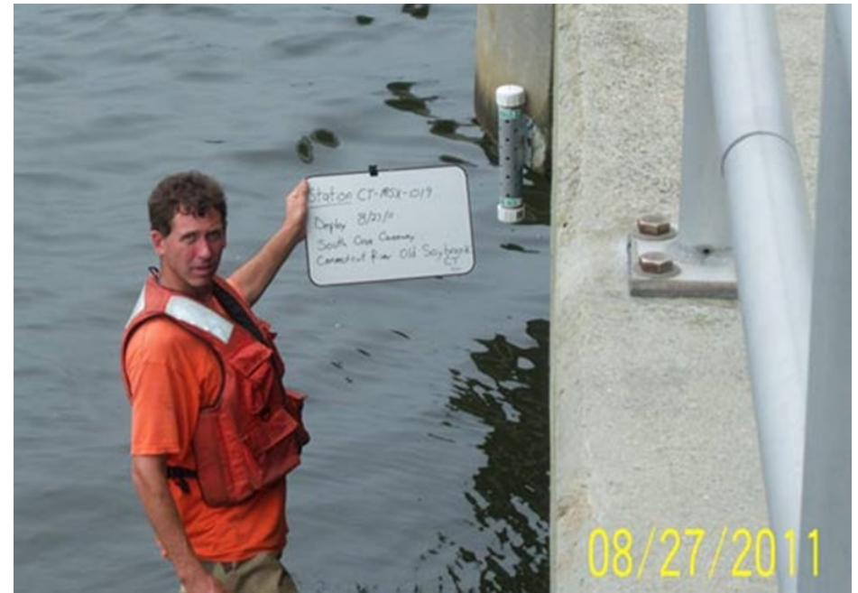
Figure 2-12: Temporary USGS Tide Gage on South Cove Causeway, measuring water levels during Hurricanes Irene and Sandy
