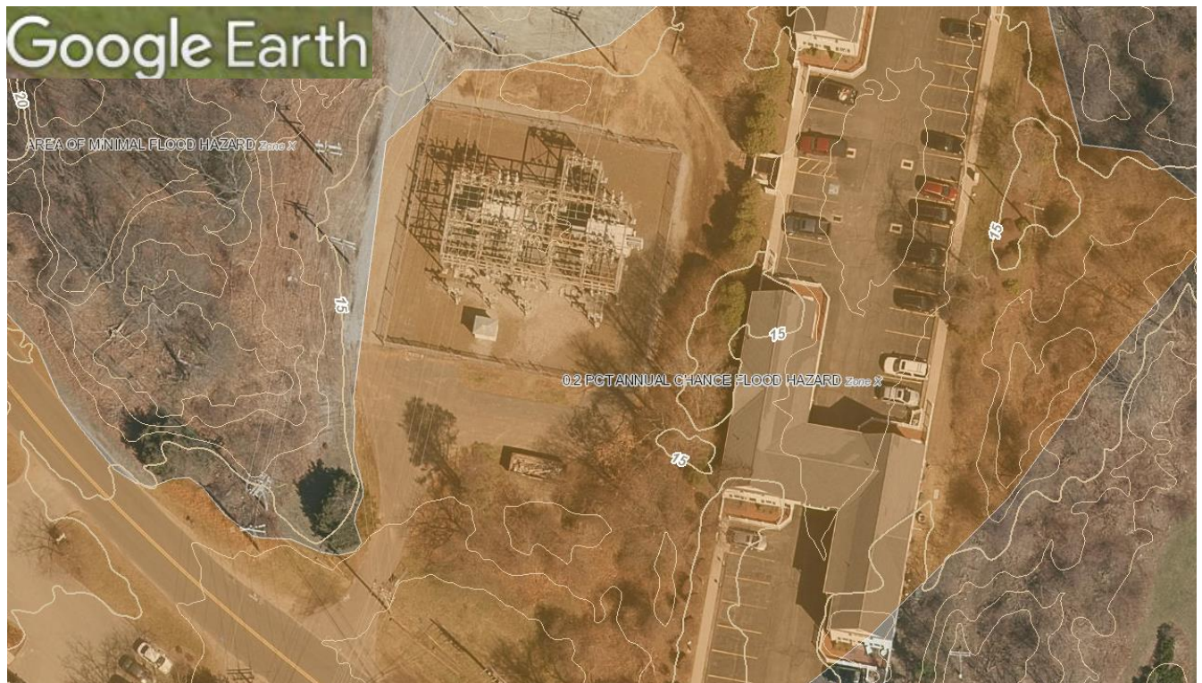
Figure 4-26 Location of Eversource Elm Street Substation relative to effective FEMA FIRM Flood Hazard Zones
