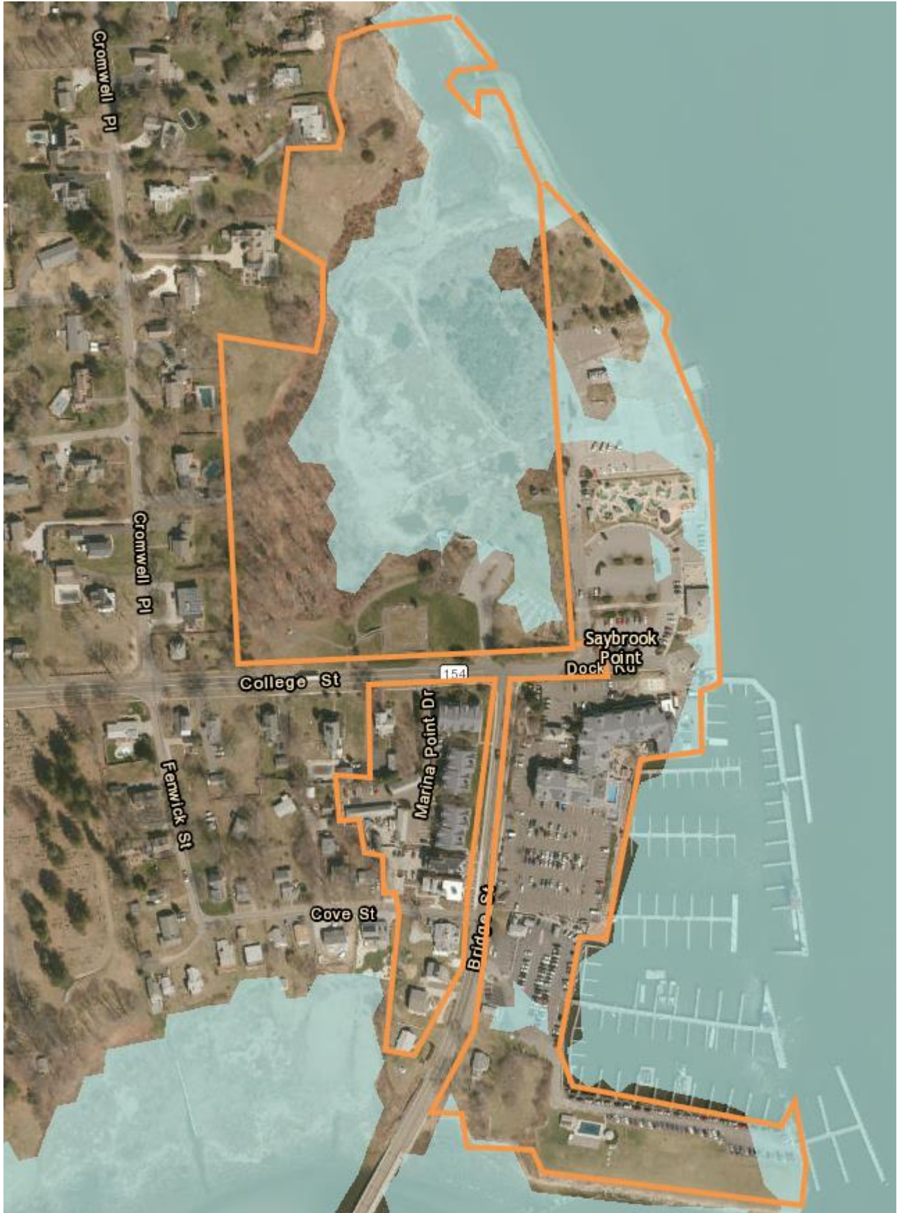
Figure 4-3 Saybrook Point SP-1 through SP-3 Districts relative to 2 year recurrence interval flood A FIRM
