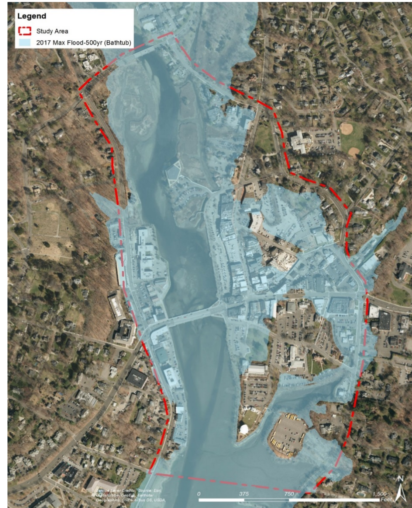
Attachment 2 Figure 13: Flood Extent in Downtown for the 2017 500-year return period (1% annual chance) peak flood inundation
