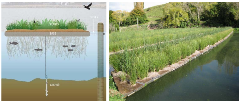
Figure 6. Generalized floating marsh schematic and deployment of interconnected marsh cells in Kauri Park, NZ.
