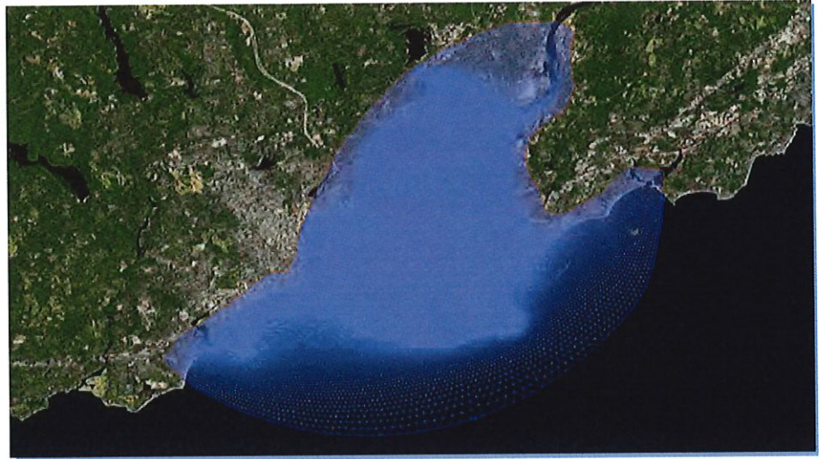
Figure 2.1 GZA High Resolution Computer Model Mesh
