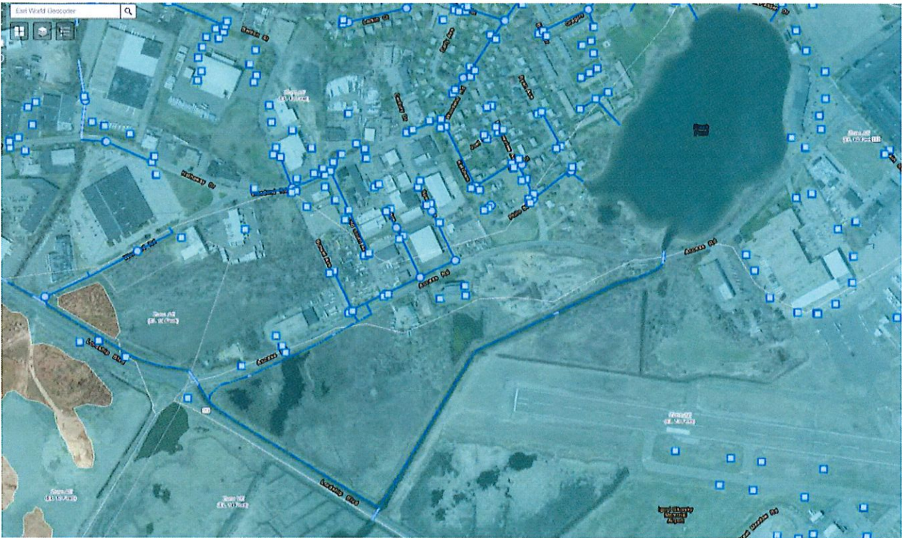
This figure indicates the effective FEMA FIRM limits of inundation and Base Flood Elevation. Existing storm drains, manholes and catch basins and area ground surface elevations also indicated.
