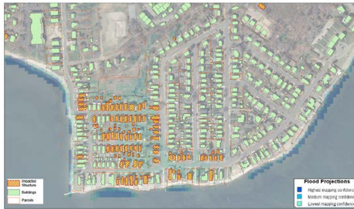
Point Beach 2020s High Tide Conditions 0 125 250 375 500 Feet Dikes and Floodwalls not constructed. All homes elevated to allow frequent flooding. Stormwater systems upgraded minimally, neighborhood drains naturally at low tide. Roadways upgraded and maintained to be floodable.
