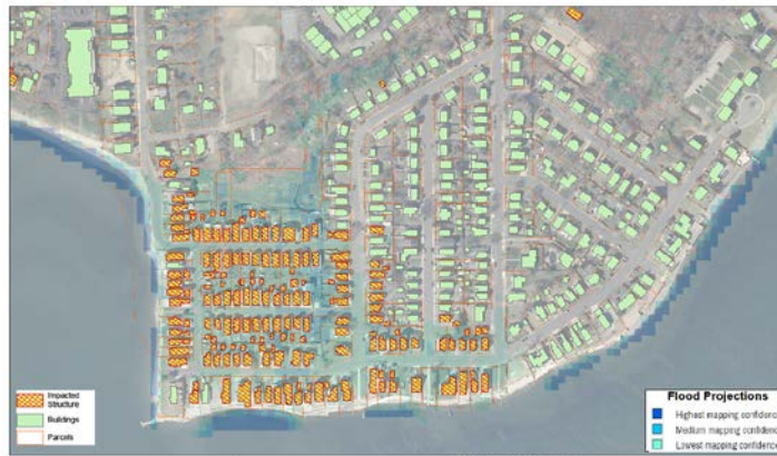
Point Beach 2030s High Tide Conditions 0 125 250 375 500 Feet Dikes and Floodwalls not constructed. All homes elevated to allow frequent flooding. Stormwater systems upgraded minimally, neighborhood drains naturally at low tide. Roadways upgraded and maintained to be floodable.
