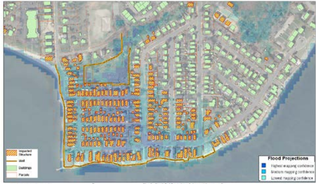
Point Beach 2020s Category 2 Storm Conditions Floodwall installed & maintained along existing seawalls. All homes elevated to allow surge flooding. Stormwater systems upgraded to prevent surcharge, and pump water against higher base level during high tides. Approximately 188 homes protected against high tide through the 2080s. "Dry Except During Storm Surge"
