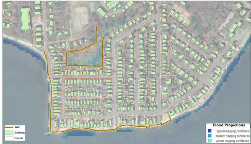
Point Beach 2080s Daily High Tide Conditions Floodwall installed & maintained along existing seawalls. All homes elevated to allow surge flooding. Stormwater systems upgraded to prevent surcharge, and pump water against higher base level during high tides. Approximately 188 homes protected against high tide through the 2080s. "Dry Except During Storm Surge"
