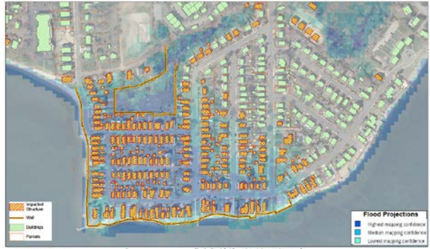
Point Beach 2080s Category 2 Storm Conditions Floodwall installed & maintained along existing seawalls. All homes elevated to allow surge flooding. Stormwater systems upgraded to prevent surcharge, and pump water against higher base level during high tides. Approximately 188 homes protected against high tide through the 2080s. "Dry Except During Storm Surge"
