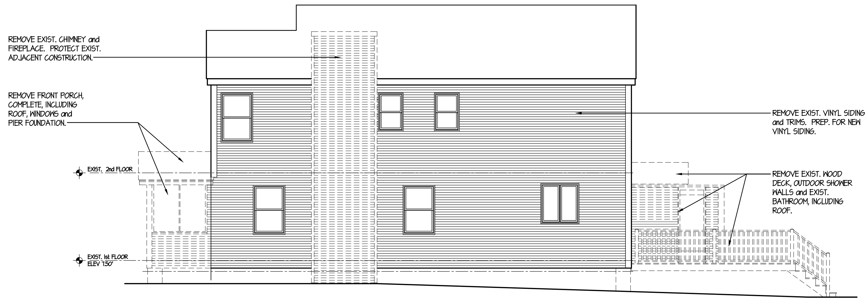
6 DEMOLITION - EAST ELEVATION
