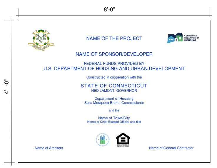
SIGN PANEL: 3/4" MDO-EXT-APA PLYWOOD SUPPORTED WITH (2) 4X4 TREATED WOOD COLUMNS AND SECURED 4' INTO GRADE. TOP OF SIGN AT 8'-0" ABOVE GRADE.
