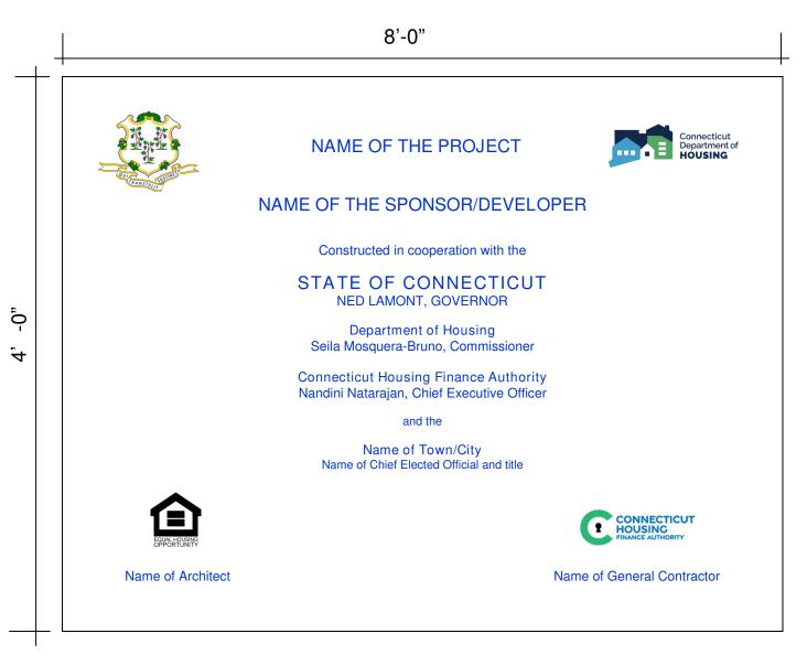
SIGN PANEL: 3/4" MDO-EXT-APA PLYWOOD SUPPORTED WITH (2) 4X4 TREATED WOOD COLUMNS AND SECURED 4' INTO GRADE. TOP OF SIGN AT 8'-0" ABOVE GRADE.
