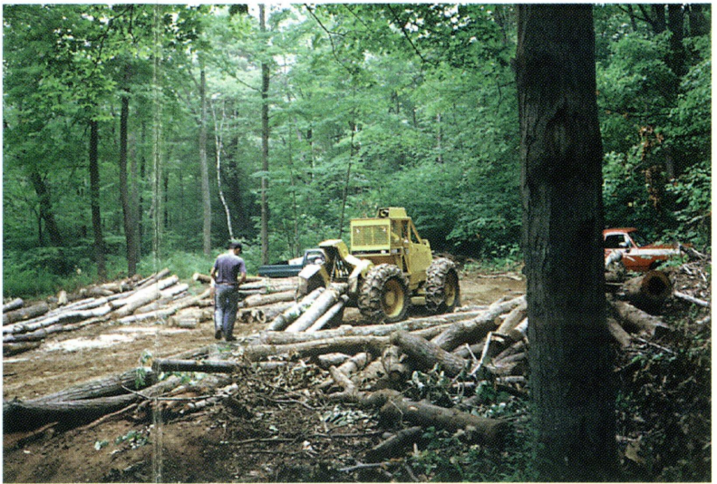
A skidder drops a load of logs in a landing area for trucking.
