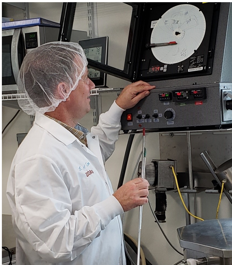
Connecticut Department of Agriculture Milk Safety Division representative, James Allyn conducting tests on a vat pasteurizer at one of Connecticut's cheese manufacturing facilities.
