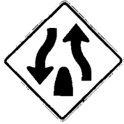
DIVIDED HIGHWAY ENDS
