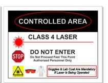
1.5.3. **Danger Class 4 Laser Safety Check** sign shall be displayed over the laser warning sign which will be illuminated when the laser is in use. The warning sign shall be on the exterior wall of the Controlled Area entrance way.
