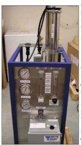
A complete reverse osmosis system consists of a RO module, a storage tank, and a separate faucet. The module contains a semi-permeable membrane that allows water to selectively pass through and collect in the storage tank. The contaminants being treated by the RO unit are rejected and then washed off the membrane into a waste stream.
