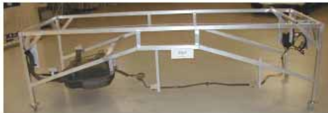
Typical Test Rig for CRC E-65 Permeation Study.
