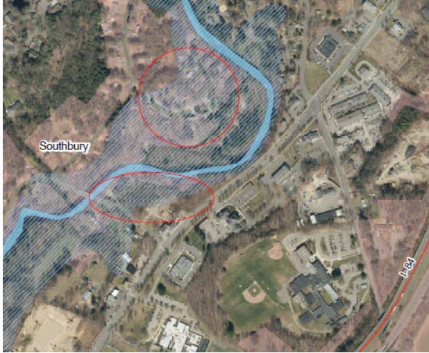
Vulnerable neighborhoods are circled in red, with the blue crosshatch indicating the FEMA flood hazard area.
