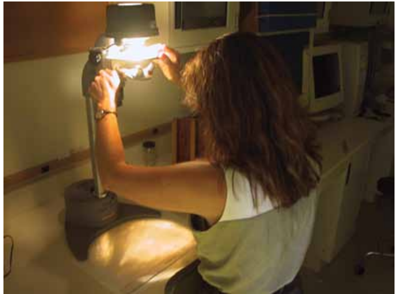
To make accurate measurements of a fish's growth, scales or bones are magnified with a specialized projector so the annual growth rings are easier to see, measure, and count.
