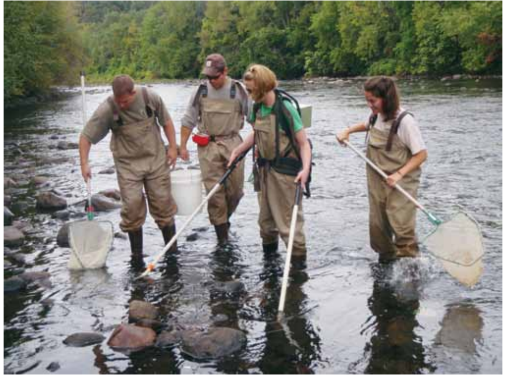
Electrofishing is a widely used method for the non-lethal collection of fish community data.
