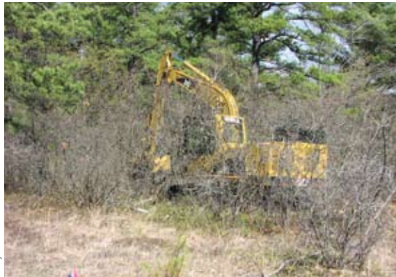
Figure 31 (top). A hydro-ax cuts down 10 acres of mature alder to create regenerating habitat for New England cottontails.
