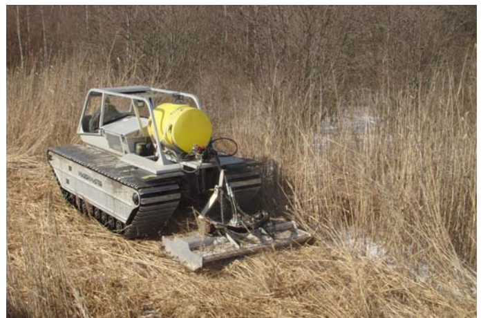
Mowing dead Phragmites stems with an amphibious Marsh Master and deck mower. Photo courtesy of Kurt Ehrhart, Innovative Mosquito Management, LLC.
