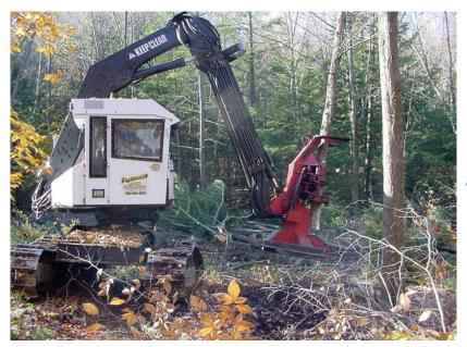
Figure 6. Feller-Buncher used in the treatment.
