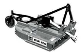
Make/ModelBushHog 285ManufacturerBushHogPreferred Prime MoverTractor 30 hp or greaterAttachment Mount3 pt Category I hitchMaximum Treatable Material Size2 inCutting Width5 ftCutting Height1.5 – 10.5 in
