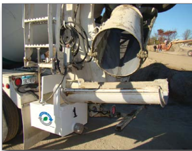
Figure 7. Chute washout box
