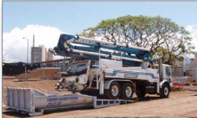
Figure 14. Pump truck using the ramp to wash out into a roll-off bin
