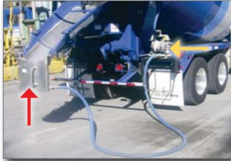
Figure 8. Chute washout bucket and pump
