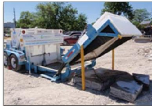
Figure 17. Delivering hardened concrete to a recycler
