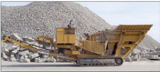
Figure 6. Crushed concrete stockpile and crusher
