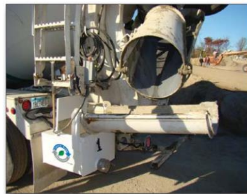
Figure 7. Chute washout box
