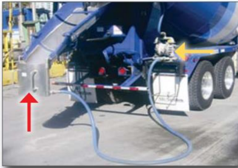
Figure 8. Chute washout bucket and pump
