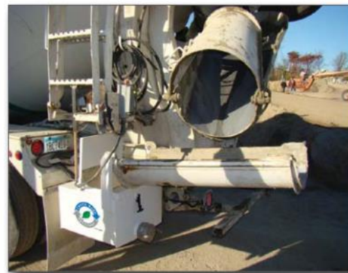
Figure 7. Chute washout box
