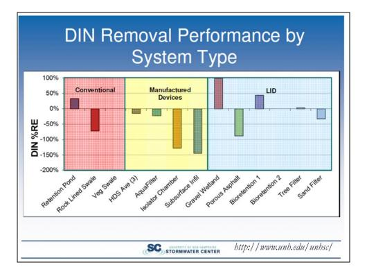
Dissolved nitrogen is difficult to remove based on the multiple water chemical conditions required for complete removal. Note that many of the devices lead to negative removal – or increasing concentrations!!! Retention ponds remove DIN while many manufactured devices release DIN. Generally those techniques involving biological methods with some retention of water will remove DIN.
