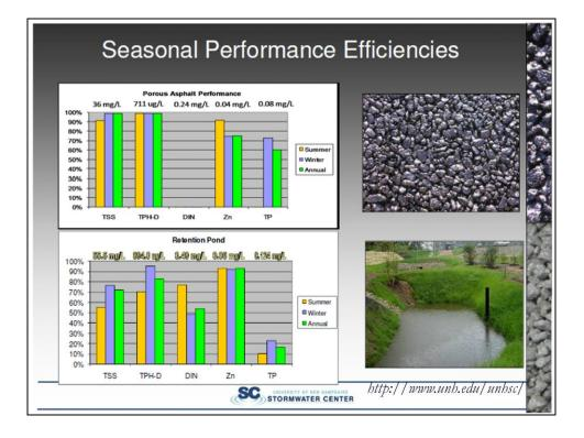
Generally porous asphalt performs well for those chemicals relating solid concentrations. Retention ponds also remove solids but achieve greater removal of DIN as well. Dissolved contaminants are more difficult to remove. Nitrogen is regulated off the dissolved portion. Metals are only regulated in their total concentration. while much lower in concentration, the dissolved portion often represents the more toxic form.
