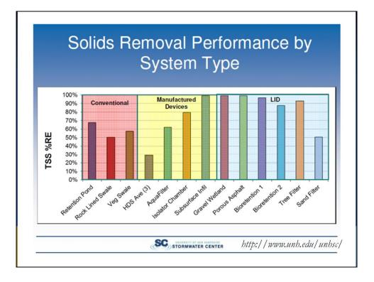
Conventional treatment of retention ponds and swales achieve 50-70% removal of solids. Some manufactured devices perform worse while others achieve almost 100%. Many LID features achieve 90-100% removal – the exception being the sand filter.
