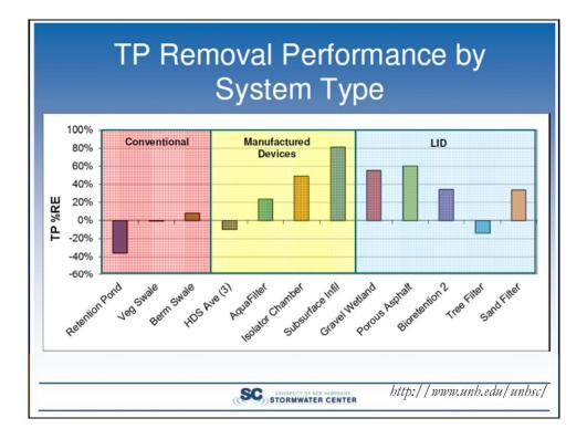
Many manufactured and LID devices remove TP due to high retention of solids. The P is attached to the solids and thus removed. Retention ponds create conditions under which P is released from the sediments and can be mobilized in the water during high flow events – hence the negative removal.
