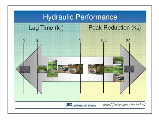
Hydraulic reduction and attenuation of the time until the peak water occurs is one performance measure. Above are a few examples: for peak reduction the porous pavement performed best with the tree filters worst. Similar for the delay to peak with the tree filter outperforming only the swale.
