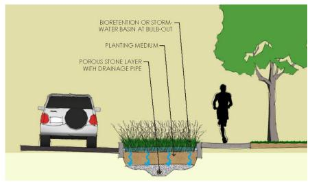
Figure 21. Typical Bioretention Bulb-out
