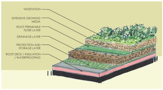
Figure 6. Typical Green Roof Design
