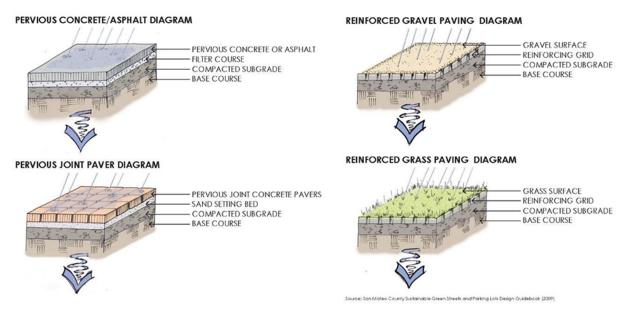
Figure 8. Diagrams of Selected Permeable Pavement Systems
