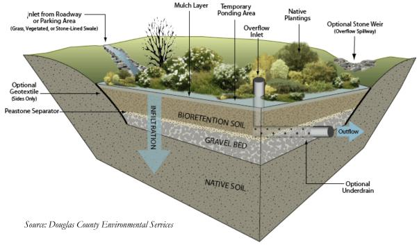
Figure 3. Typical Bioretention Design
