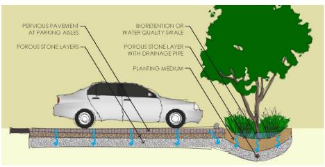
Figure 2. Typical Pervious Parking Stalls with Vegetated Swale
