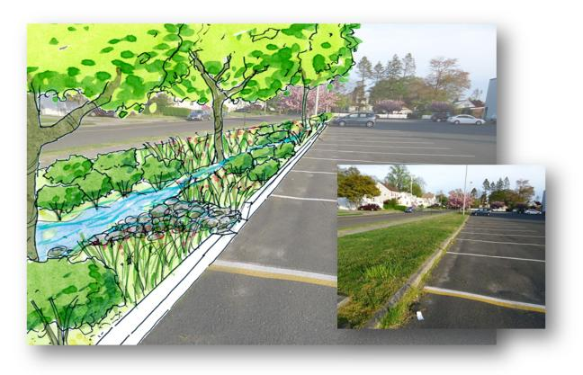
Figure 7. Before and After Concept Design for a Bioretention Area for the Parking Lot
