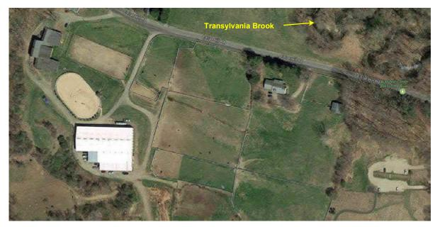
Figure 2: View of equestrian center adjacent to the start of reach Pomperaug-01. Runoff from paddock areas appears to channelize in several places and ultimately discharge to both Transylvania Brook and the Pomperaug River.
