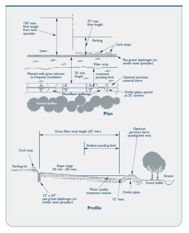
Figure 4.4: Vegetated Filter Strip Schematic. Source: CT Stormwater Quality Manual
