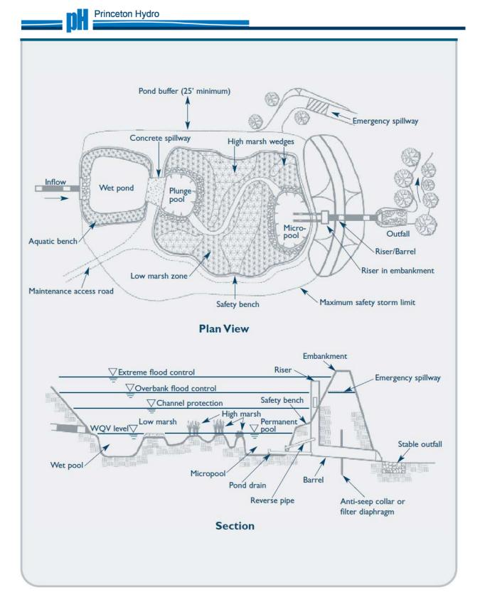
Figure 4.2: Pond/Wetland System. Source: CT Stormwater Quality Manual
