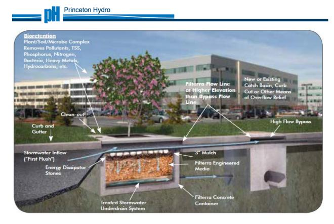
Figure 4.6: Tree Well Schematic. Source: Contech Engineered Solutions
