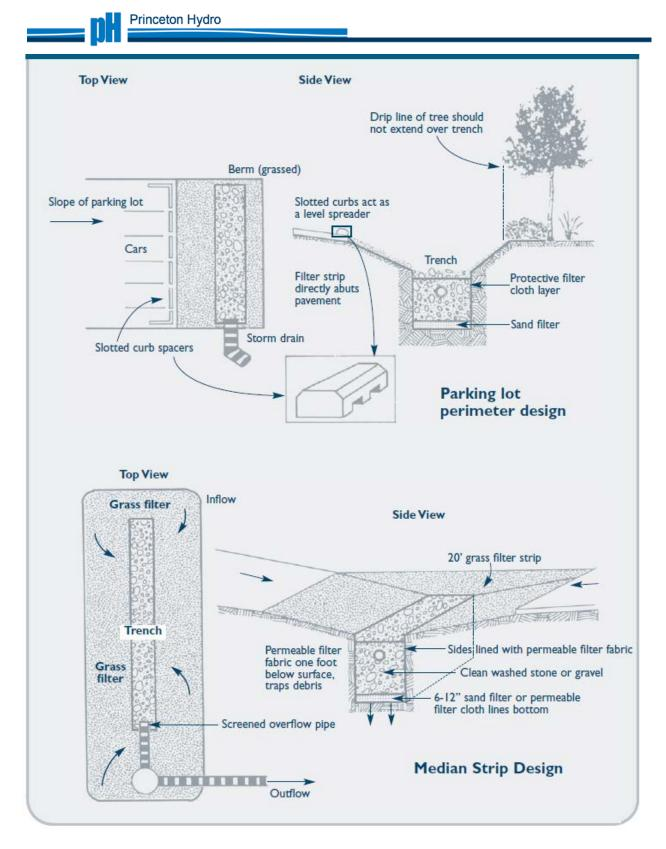
Figure 4.3: Infiltration Trench Design for Parking Lots. Source: CT Stormwater Quality Manual
