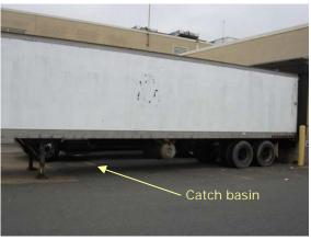
Truck loading/unloading operations at this dock occur over a stormwater catch basin, increasing the potential for oil and spills to enter the system.
