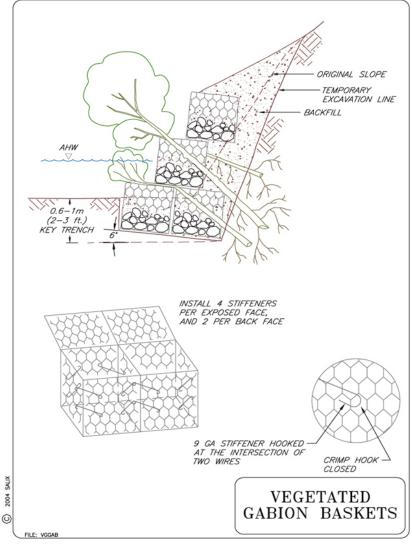
Figure 5.19: Gabion Detail
