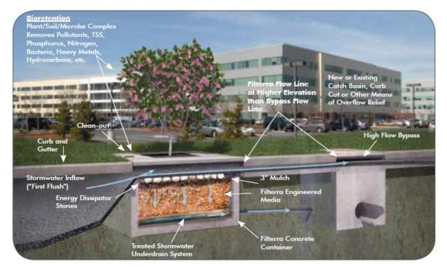
Figure 5.11: Tree Well Schematic. Source: Contech Engineered Solutions
