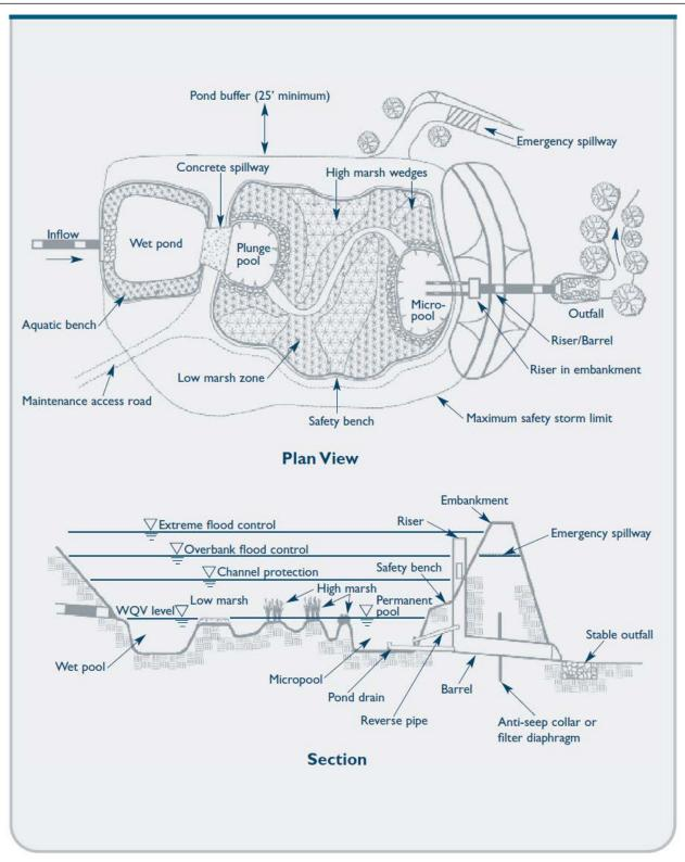
Figure 5.5: Pond/Wetland System. Source: CT Stormwater Quality Manual
