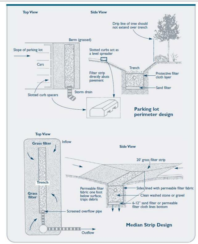
Figure 5.6: Infiltration Trench Design for Parking Lots. Source: CT Stormwater Quality Manual
