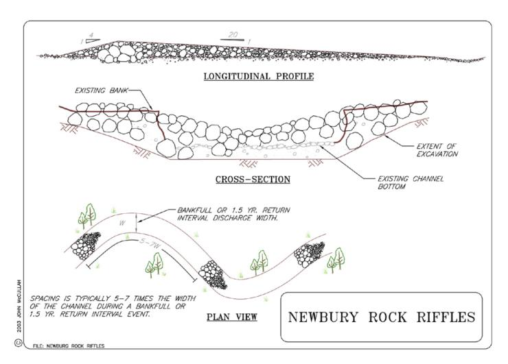
Figure 5.21: Engineered Rock Riffle Detail
