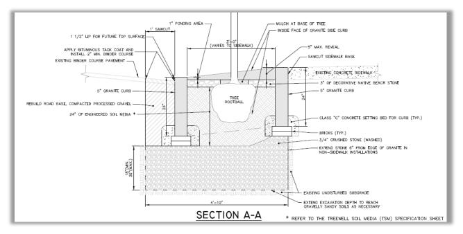
Figure 5.10: Tree Well Schematic. Source: Eastern Connecticut Conservation District
