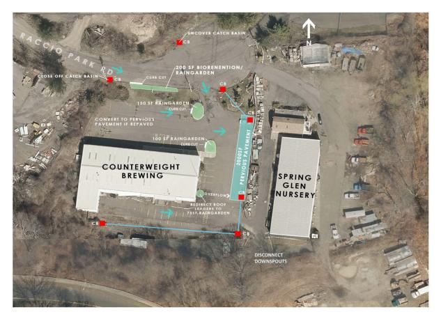
Figure 22. Proposed green infrastructure retrofits for Counter Weight Brewery and Raccio Park Road. "CB" indicates existing catch basin. Blue arrows indicate existing surface flow patterns.
