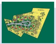
to reduce fertilizer and maintenance impacts. The access road is narrower (20 ft.) than typically allowed by ordinance and is constructed of interlocking concrete pavers that allow infiltration.
