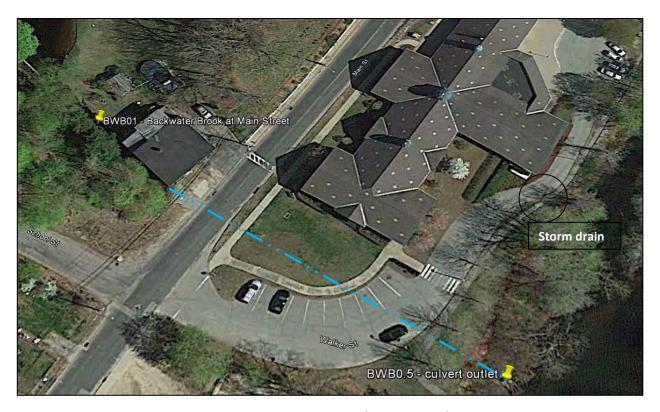
Figure 31. Culverted segment of Backwater Brook (dashed line). Approximately 250 feet of the stream is culverted under Main Street and the Thompson Public Library property.
