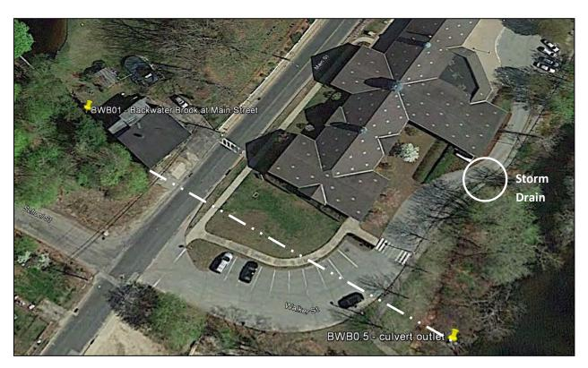
**Figure 6.** Culverted segment of Backwater Brook (dashed line). Approximately 250 feet of the stream is culverted under Main Street and the Thompson Public Library property.
