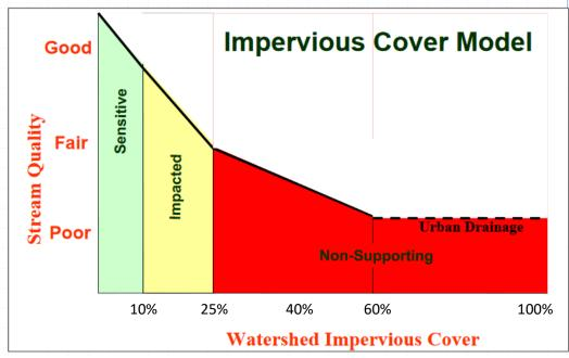
Figure 5-1. The relationship between stream quality and impervious cover in a watershed (Schueler, 1994).
