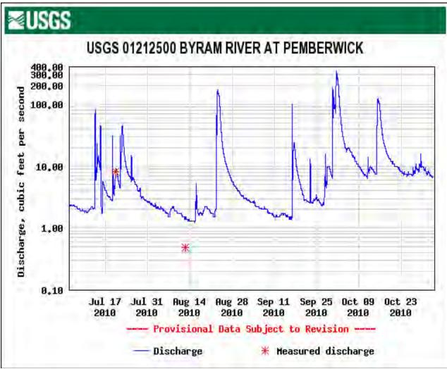
Figure 3. A representative Discharge Graph indicating the flashiness of the Byram River. Each spike corresponds to a rain event.
