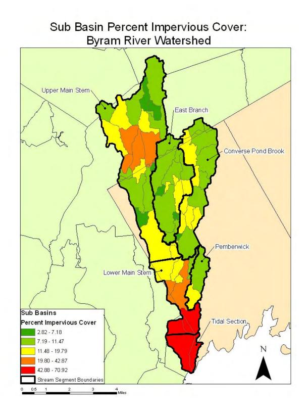
Figure 7. Byram River Watershed Percent Impervious Area for Individual Sub Basins
