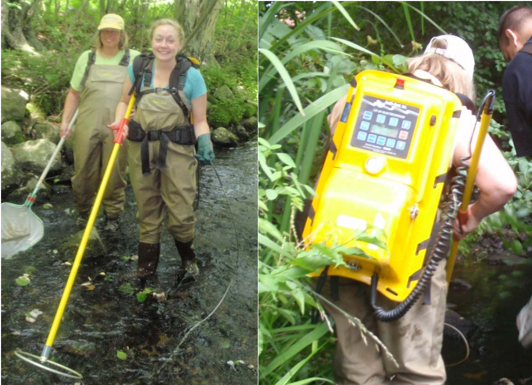
Figure 4.3. A Smith-Root backpack electrofishing unit. The black rat tail is visible in the operator's left hand and the anode (pole with ring) in her right hand. Note the red on/off switch located on the anode pole handle Note the red on/off button at the top of the unit.
