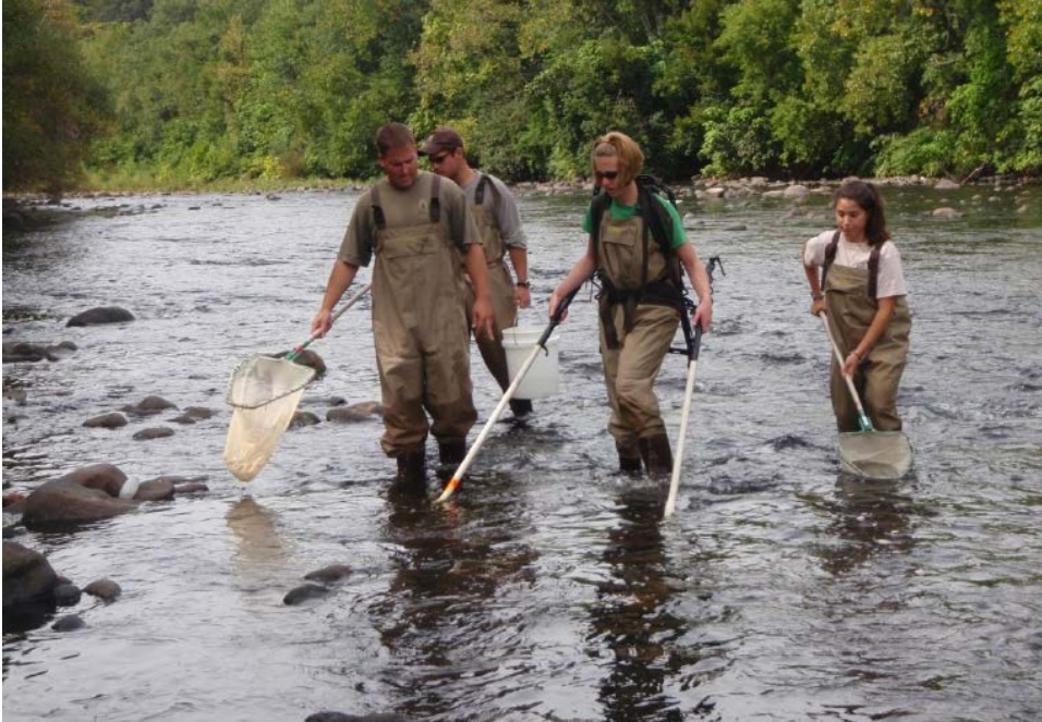
Figure 4.1. A four-person electrofishing crew operating a single backpack electrofishing unit. One individual operates the backpack (center), netters follow to the right and left of the backpack, and a crew member remains in the back with a bucket to contain stunned fish.
