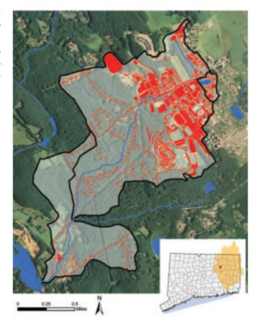
Figure 2. The Eagleville Brook watershed and its location (inset) within the state and within the Thames River major basin. Black lines depict the boundaries of the watershed and subwatersheds, blue lines represent water, and red areas depict impervious cover digitized from 2008 high-resolution imagery, that comprises the map background. The University of Connecticut campus can be seen as the concentration of impervious cover in the upper watershed.
