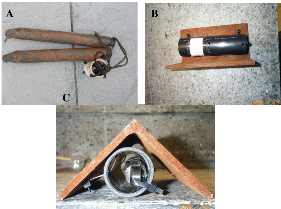
Figure 15. (A) TidbiT ® tethered to PVC housing with tie wraps and fastened to window weights with parachute cord. (B) and (C) HOBO ® Pro v2 attached to PVC housing with tie wraps and angle iron weight.
