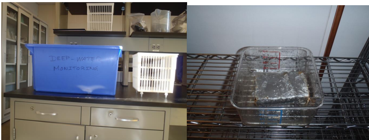
Figure 2. Required containers for an ice water bath set-up (left to right): large plastic bin, small perforated container with attached 'foot' stands, and a plastic container with a weight.
