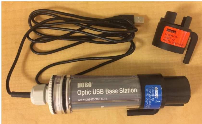
Figure 4. HOBOWare Optic USB Base Station shown with HOBOWare Pro v2 (blue, attached) and Tidbit (orange) couplers.
