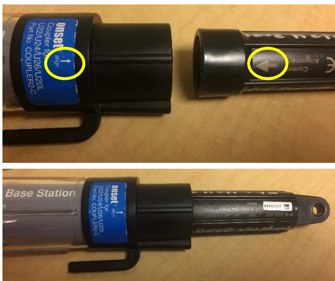
Figure 5a-b: (a; top) Coupler and logger alignment arrows (yellow circles); (b; bottom) HOBOWare Pro v2 logger successfully inserted into the coupler.
